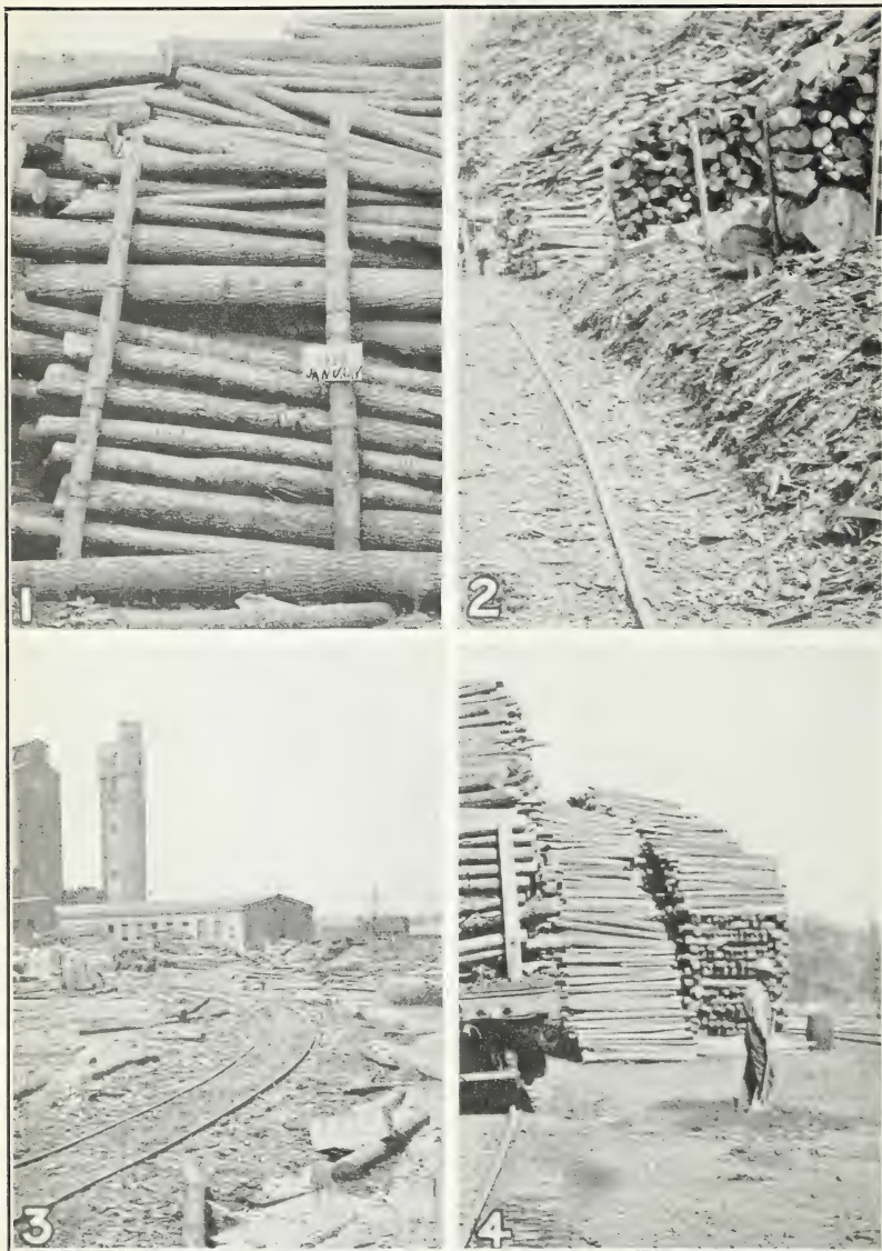
FIG. 1.—Pulp wood piles marked with date of arrival at the mill, to be used in rotation FIG. 2.—Bark accumulation resulting from the hand peeling of hardwoods, a source of infection to wood piled on it. It was several feet thick over the entire yard FIG. 3.—A storage yard on swampy ground. Pulp and pulp wood can not be stored under such conditions without heavy loss. Certain portions of the yard were being raised several feet with barker waste, surfaced with cinders. Earth and cinders would serve the purpose much better FIG. 4.—Wood yard surfaced with cinders and located on a well-drained slope. The company recognizes the value of cleanliness and employs a crew to rake up and remove all accumulated bark and rotten wood. Workman "spudding" out grass and weeds and leveling the cinders. Wood is not usually stored longer than a year, and there is no appreciable loss from decay
